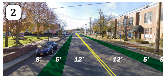
(Parking, bike lane, buffer, travel lane x2, buffer, bike lane, parking)
